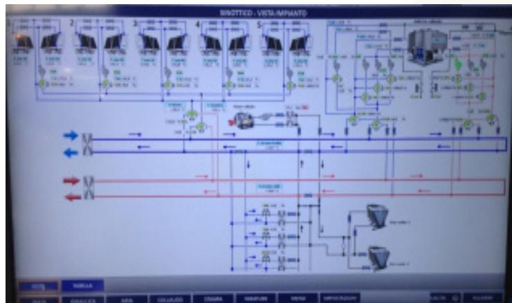
"Galleon" Laboratory permits the performances measurement of water cooled chillers / heat pumps up to 1.500 kW and air cooled chillers up to 1.200 kW
